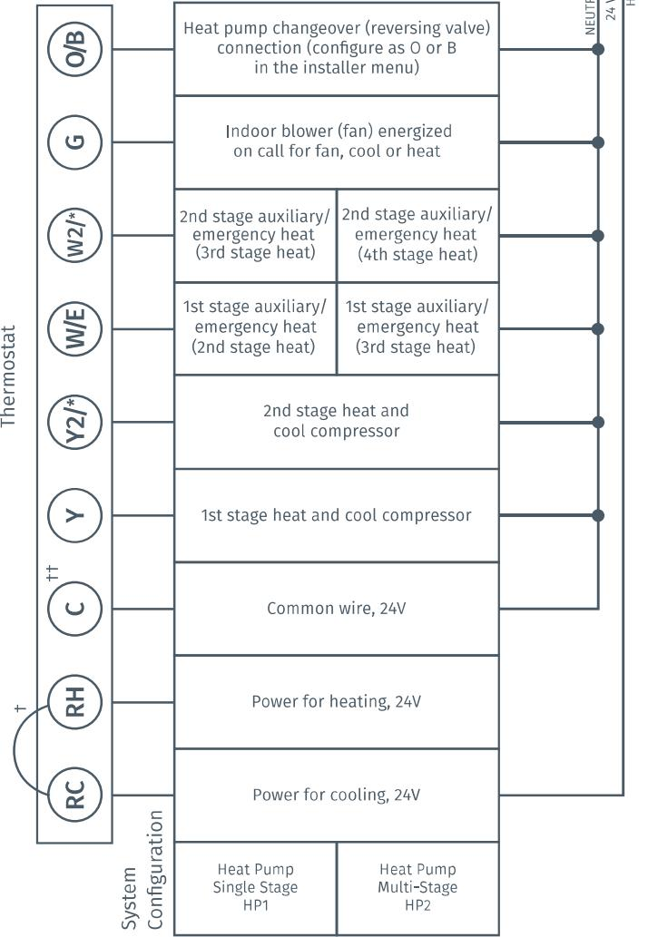
\*Internal jumper between RC and RH, located on back of thermostat.
