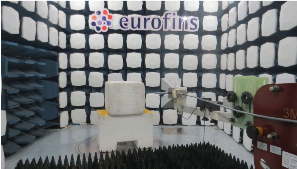
Picture 1 Radiated Emission Test Setup
