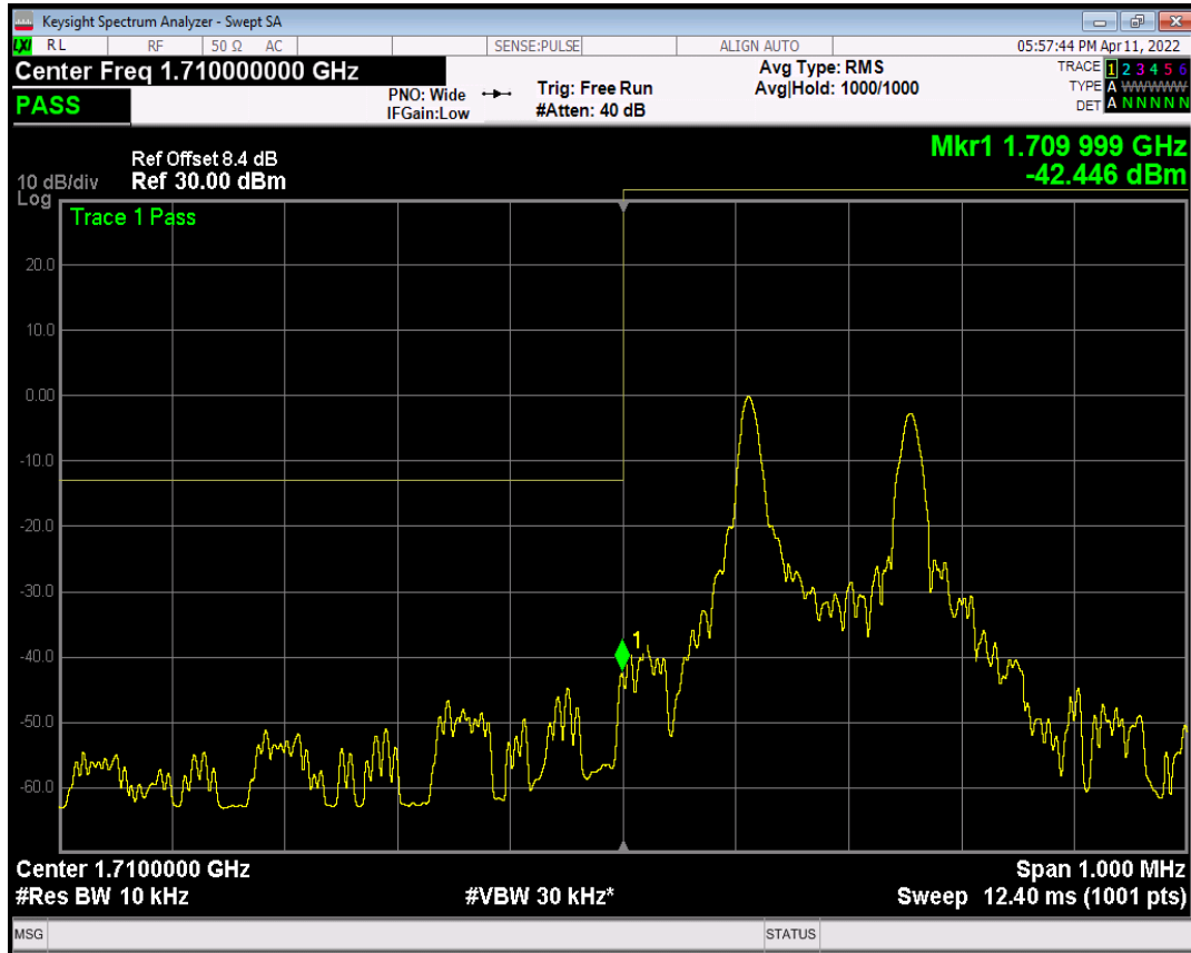
Band4 QPSK Channel=19952 nTones=1@0 Spacing=3.75kHz
