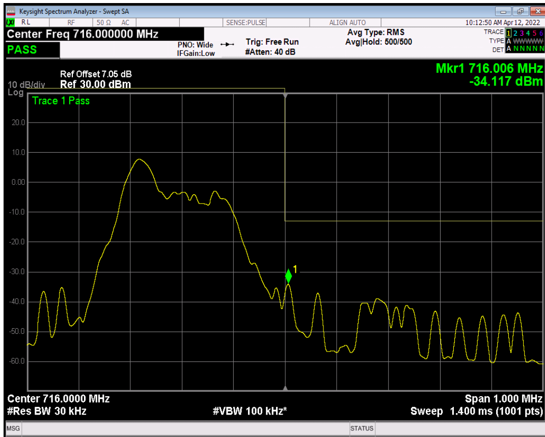
Band13 BPSK Channel=23182 nTones=1@0 Spacing=3.75kHz
