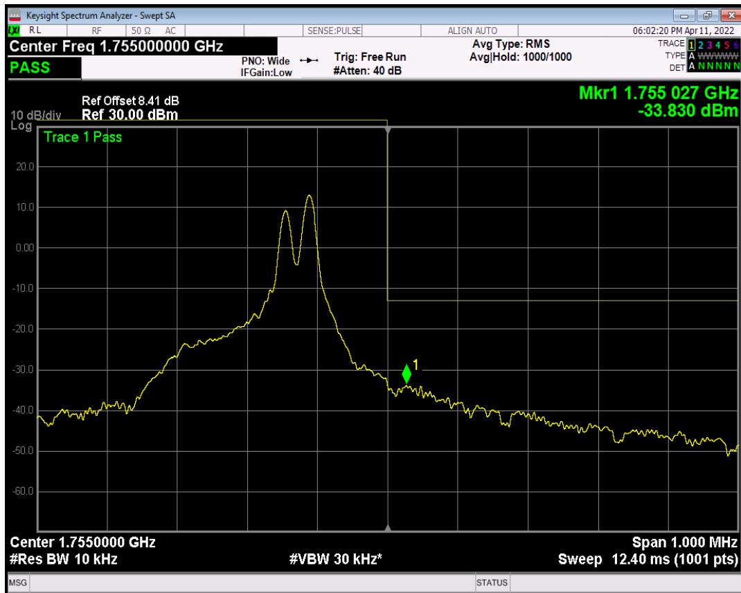
Band4 QPSK Channel=20398 nTones=1@47 Spacing=3.75kHz
