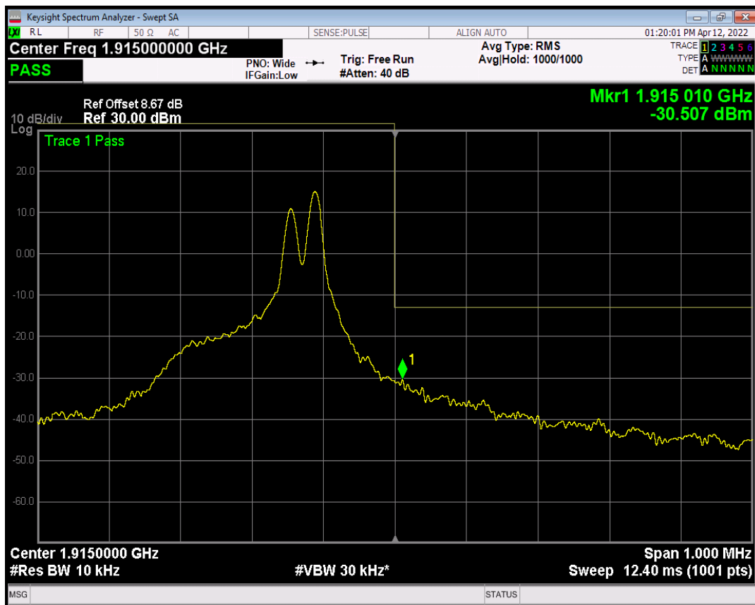
Band25 QPSK Channel=26688 nTones=1@47 Spacing=3.75kHz
