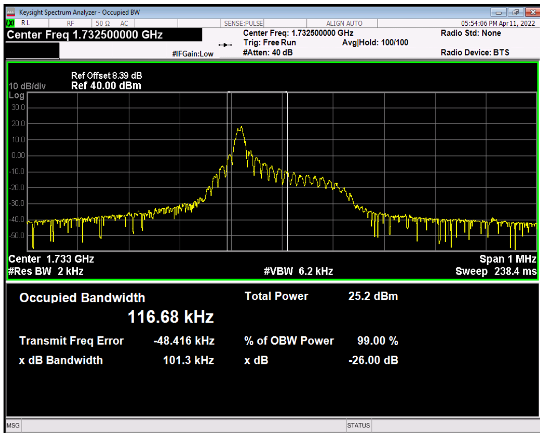
Band4 QPSK Channel=20175 nTones=1@0 Spacing=15kHz
