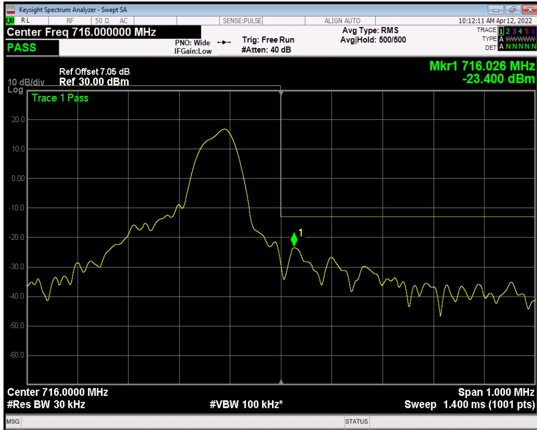
Band12 QPSK Channel=23178 nTones=1@47 Spacing=3.75kHz
