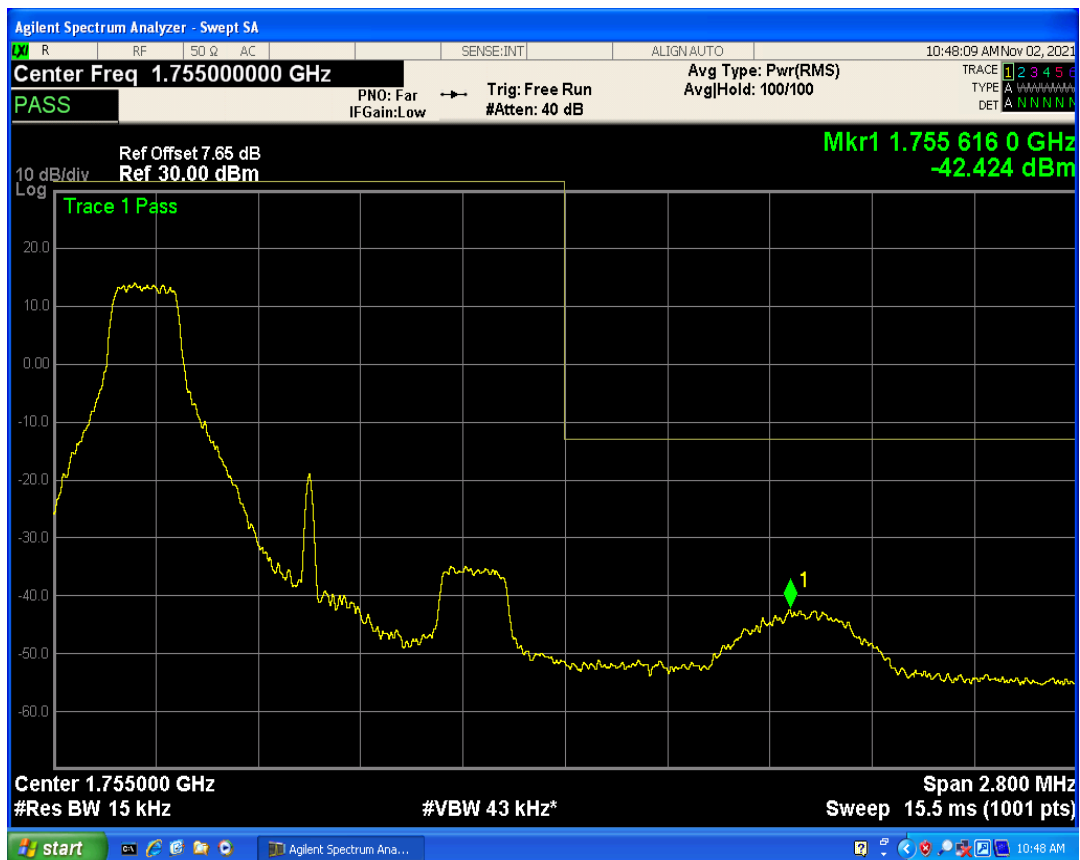
Band4 QPSK BW=1.4MHz Channel=19957 RB Size=6 Position=#0
