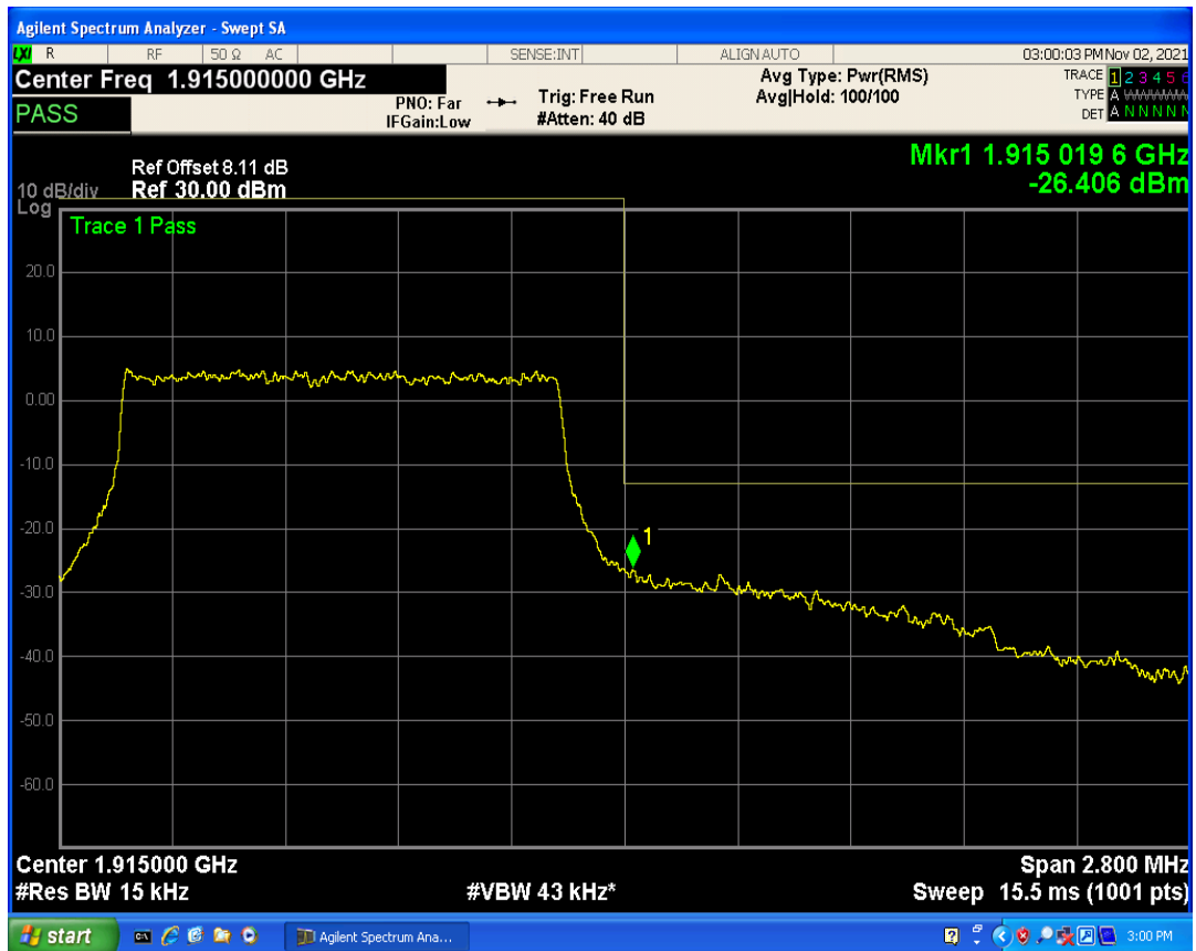
Band25 QAM16 BW=1.4MHz Channel=26047 RB Size=1 Position=#0
