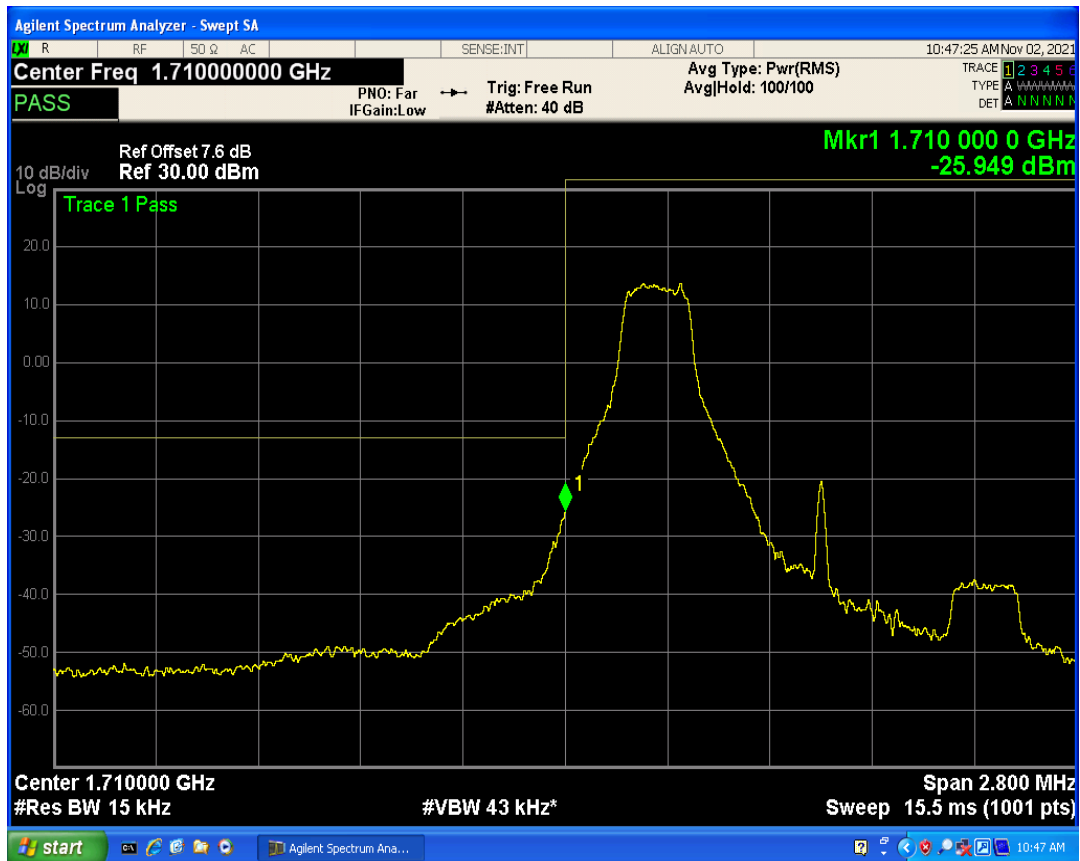
Band4 QPSK BW=1.4MHz Channel=19957 RB Size=1 Position=#Max
