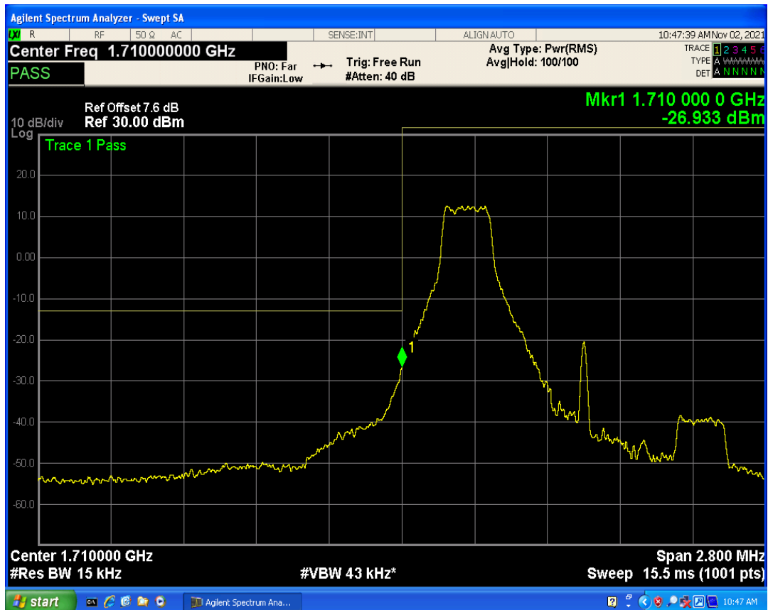
Band4 QAM16 BW=1.4MHz Channel=19957 RB Size=1 Position=#Max
