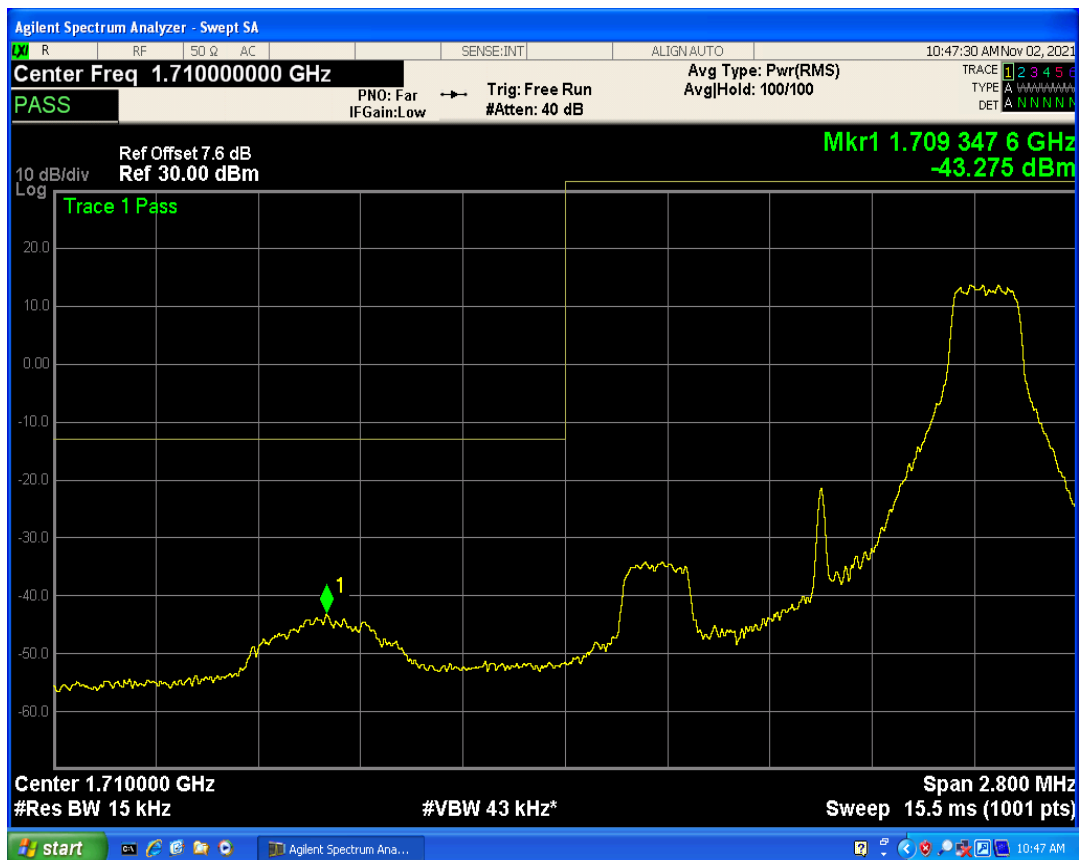
Band4 QPSK BW=1.4MHz Channel=20393 RB Size=6 Position=#0
