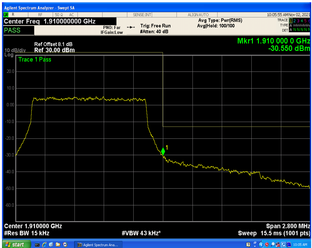
Band2 QPSK BW=1.4MHz Channel=18607 RB Size=6 Position=#0
