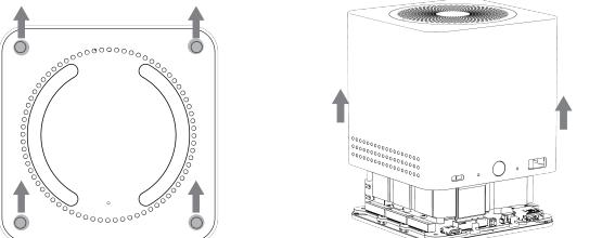
② Peel off the silicone protective film from the location where you intend to install the hard drive, remove the screws, and install the hard drive.
