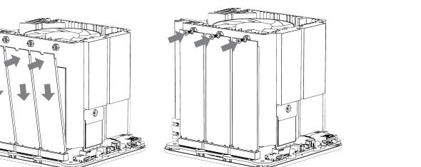
④ Put back the protective cover, tighten the four screws, and reinsert the silicone plugs.
