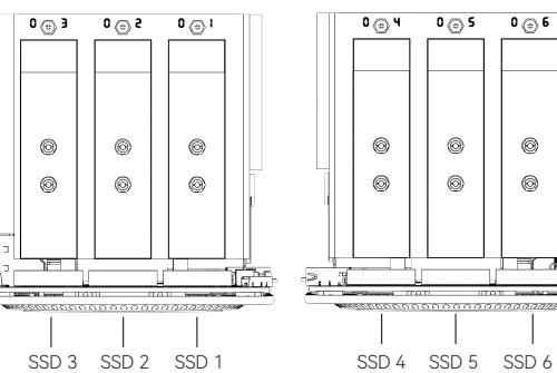
! Note: The default OS is pre-installed on the onboard eMMC. To install it on an SSD, it is recommended to use system drive 4, which runs at PCIe 3.0 x2 speed and is compatible with SATA3 hard drives. Drives 1, 2, 3, 5, and 6 function as storage drives, operating at PCIe 3.0 x1 speed.
