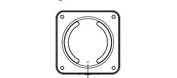
⚠ Note: Power indicator light 1 glows white when the ME mini is in operation; Power indicator light 2 glows orange when the ME mini is in sleep mode.
