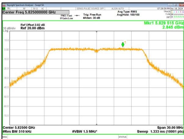
(802.11a) PSD plot on channel 165
