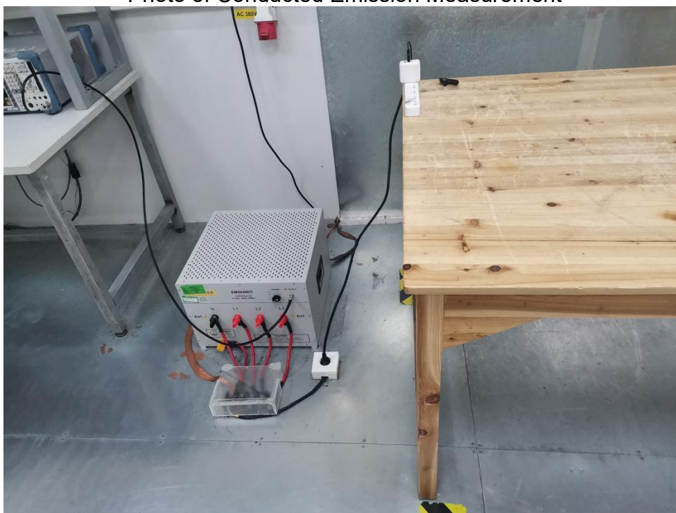
FCC ID: 2A4I9-ISBEV9 Photo of Conducted Emission Measurement
