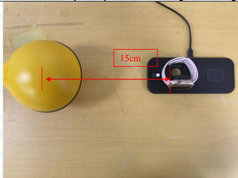
**H-Field Strength- 15 cm****Test Position E - Exposure photo from top surface**
