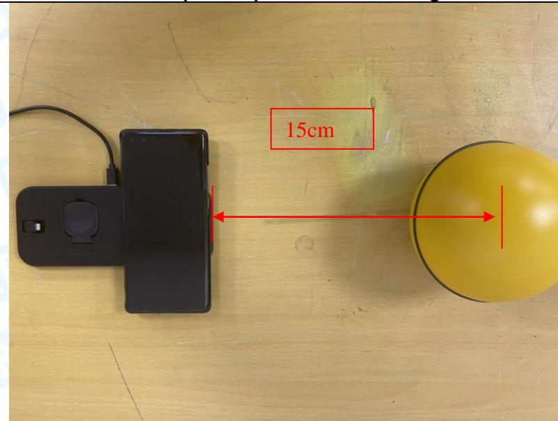
**H-Field Strength-15cm****Test Position C - Exposure photo from side edge surface-Front**
