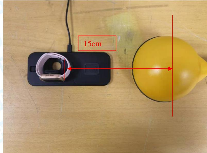
**H-Field Strength-15cm****Test Position C - Exposure photo from side edge surface-Front**
