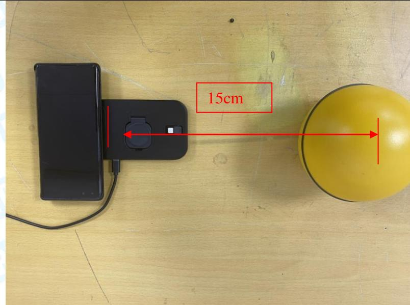
**H-Field Strength- 15 cm****Test Position E - Exposure photo from top surface**
