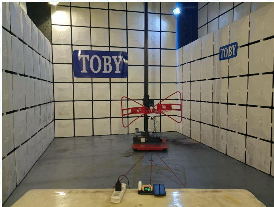
Photo of Setup for Radiated Emission (9KHz-30MHz)
