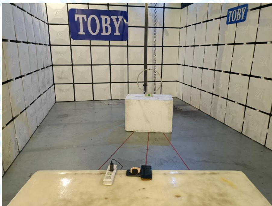
Photo of Setup for Radiated Emission (9KHz-30MHz)
