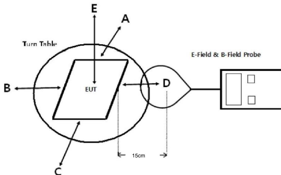
Note: The aggregate H-field strengths at 15 cm surrounding the device and 20 cm above the top surface.
