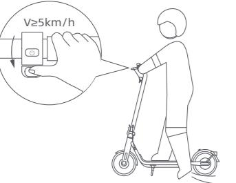
EN Step on the deck with one foot, and slowly kick off the other on the ground. When the scooter starts to coast, put both feet on the deck and gently press the accelerator.
