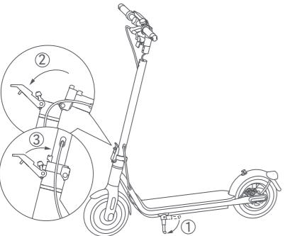
EN Put down the kickstand, and hold up the stem until it is completely in an upright position. Then push the quick release lever inward to the end.
