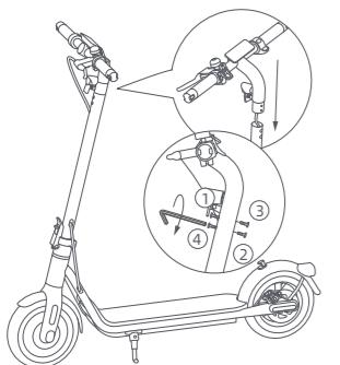
EN Install the handlebar onto the stem, and make sure to install the handlebar in the correct direction. Follow the number order as illustrated to pre-tighten the four screws with the included Allen key. Make sure the handlebar is correctly installed and then tighten the screws thoroughly.
