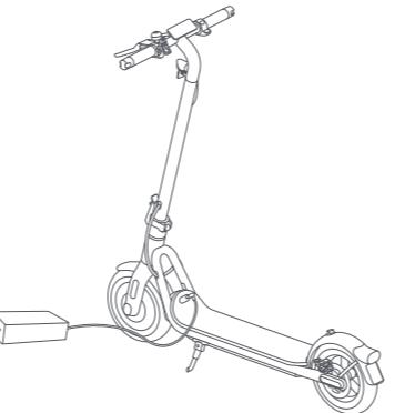
EN Charge your scooter indoors, and never expose it to rain. The scooter is fully charged when the LED on the battery charger changes from red to green.
