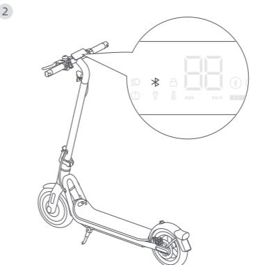
EN Power on the scooter, a blinking Bluetooth icon indicates the scooter is waiting for a connection.
