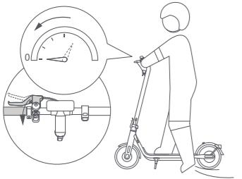
EN Release the accelerator to slow down, and squeeze the brake lever for a sudden brake.
