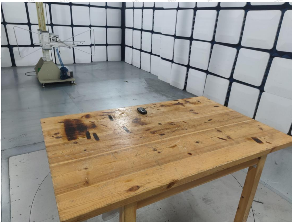
Photo of Radiation Emission Test
