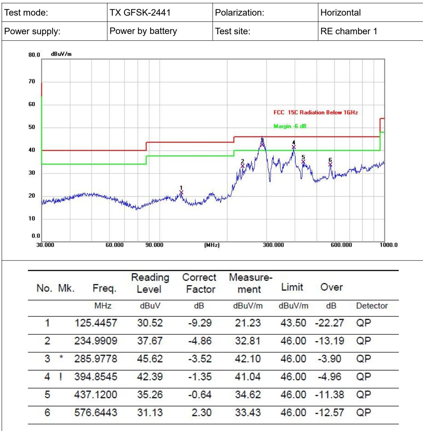
**Radiated emissions between 30MHz – 1GHz**
