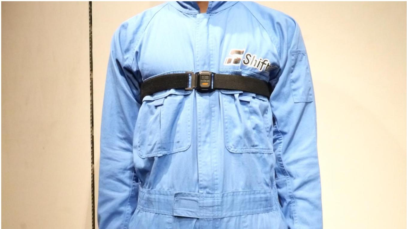
Place the chest sensor as high as possible, and the hip sensor as close to the pelvis as possible.
