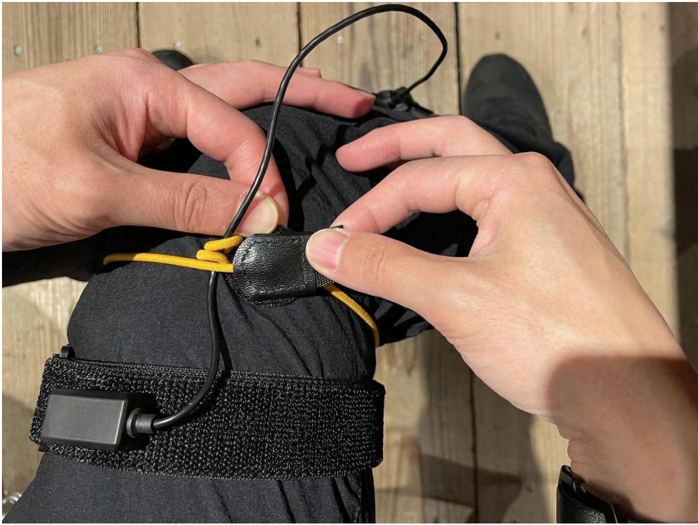
\*The leg sensors have a distance sensor to detect the movement of the ankle. Ankle motion detection may malfunction if objects such as trouser hems, shoelaces, or slippers are between the top of the foot and the sensor.
