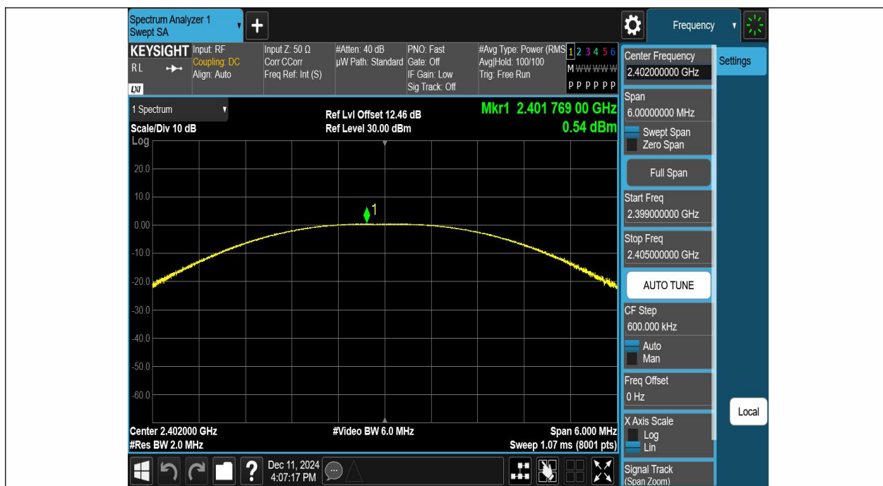
2.4G DTS MIMO-Ant1-2402-PASS
