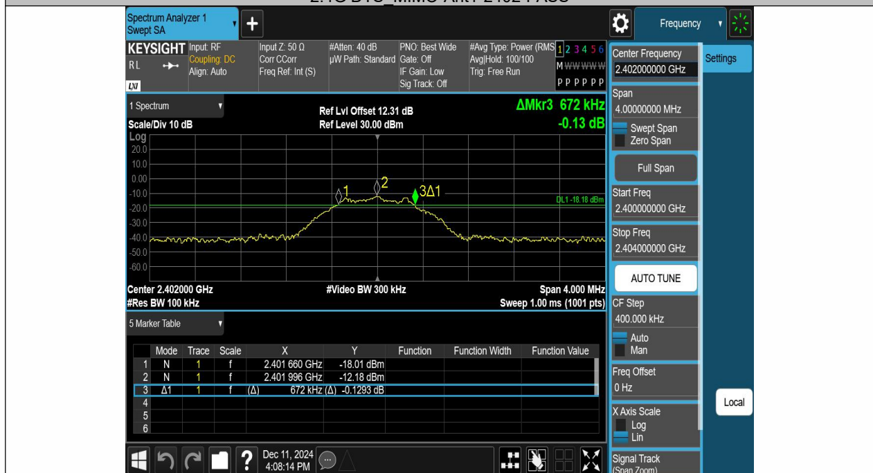
2.4G DTS MIMO-Ant2-2402-PASS
