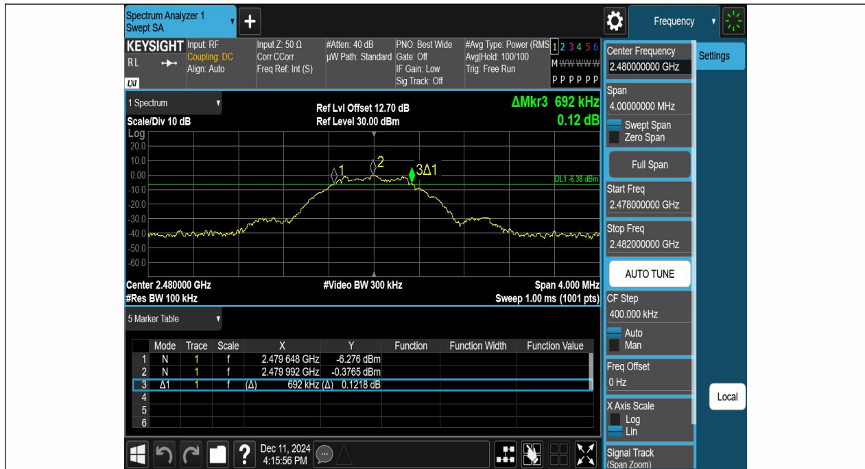
2.4G DTS MIMO-Ant1-2480-PASS
