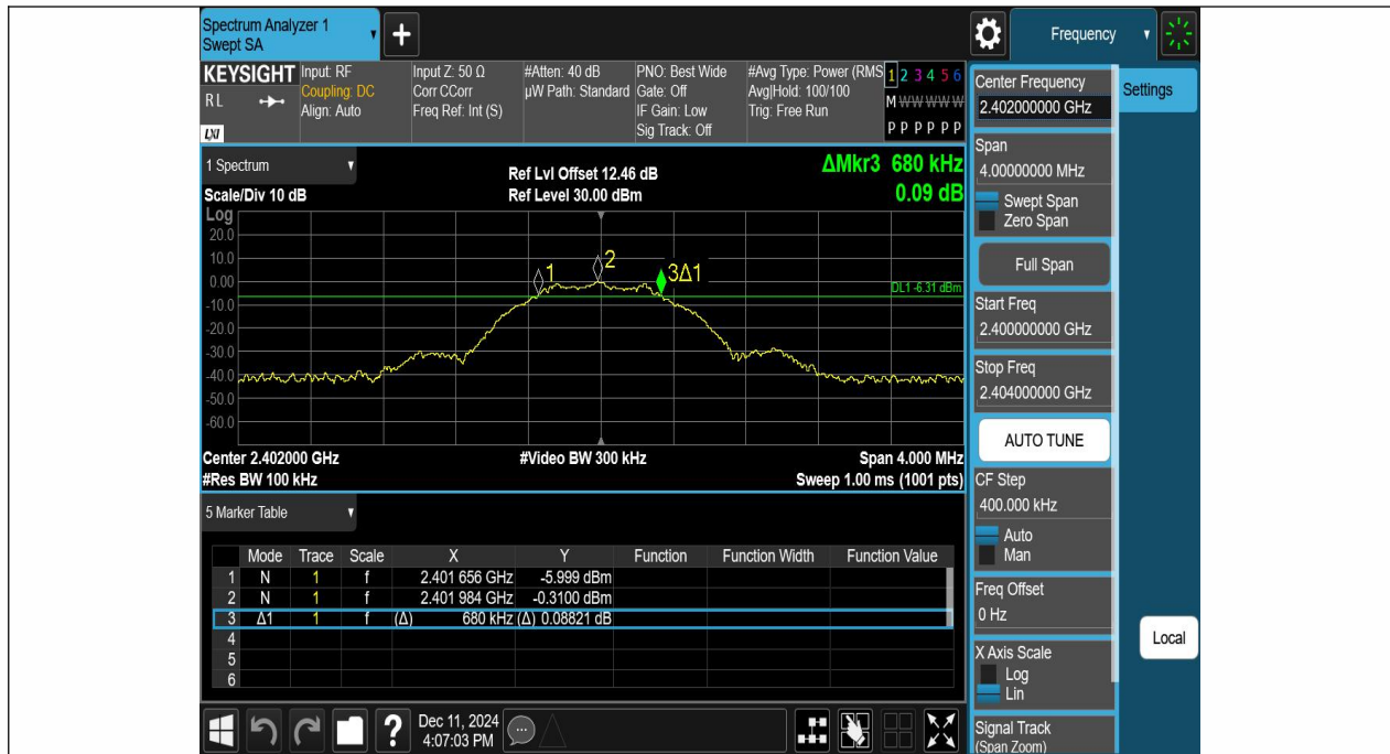
2.4G DTS MIMO-Ant1-2402-PASS
