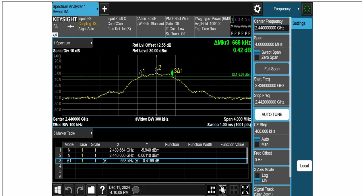
2.4G DTS MIMO-Ant1-2440-PASS
