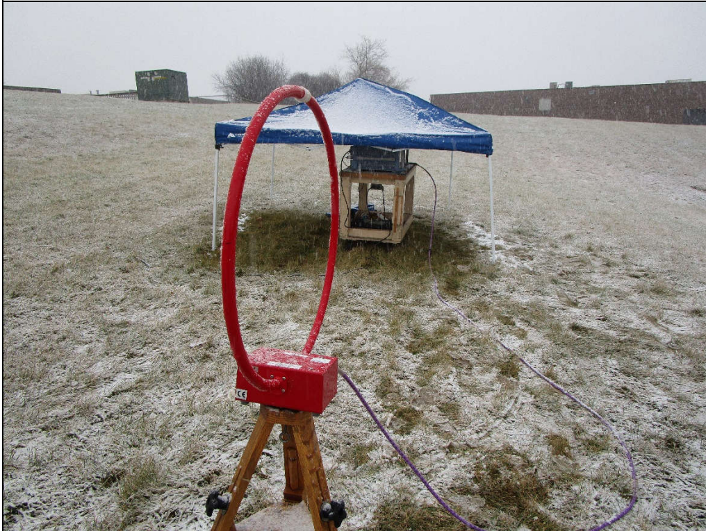
Test Setup for Radiated Spurious Emissions – 150kHz – 30MHz Y-Axis Polarization
