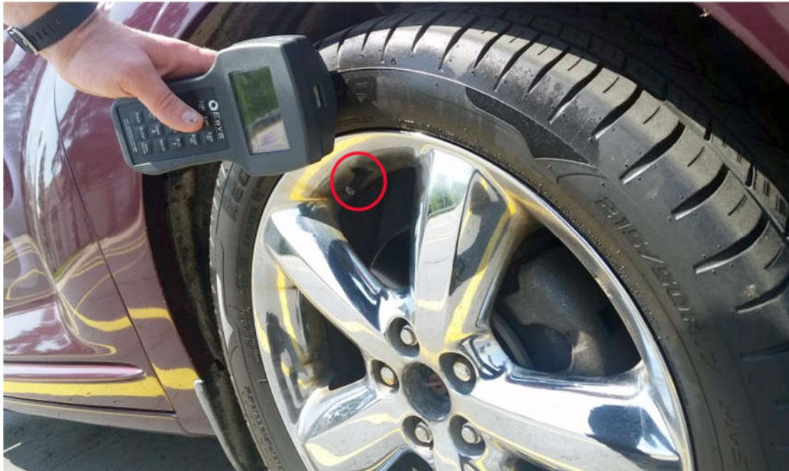
Press the corresponding wheel location button to initiate a read. It is important to press the corresponding wheel location, since this associate the stems serial number to that wheel. Once the stem read completes, the serial number and pressure will be displayed.
