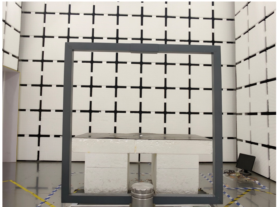
Radiation Emission Test Setup (Below 30MHz)
