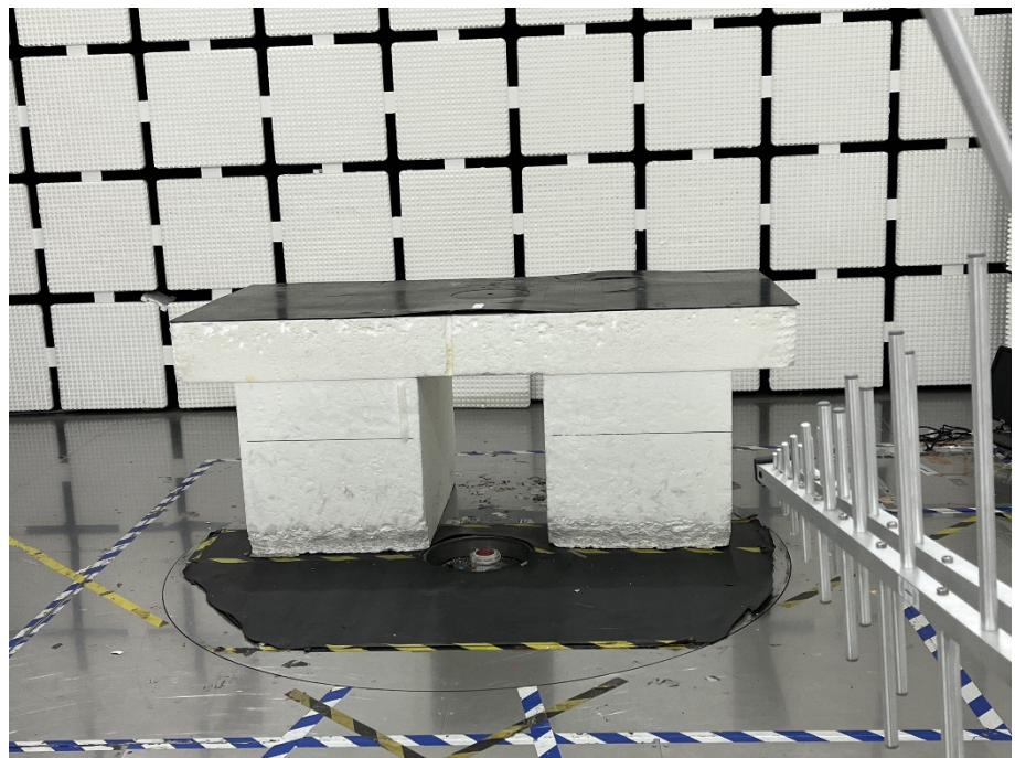
Radiation Emission Test Setup (30MHz to 1GHz)
