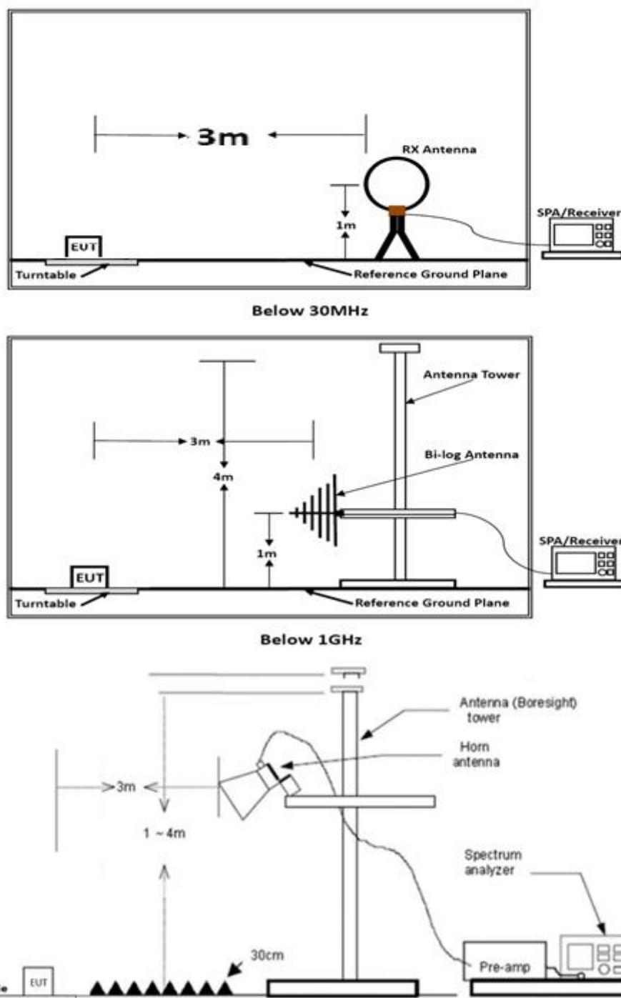
Above 18 GHz shall be extrapolated to the specified distance using an extrapolation factor of 20 dB/decade from 3m to 1m.
