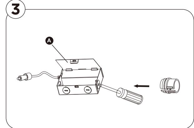
3. Carefully remove the knock-out with a screw driver or punch.
