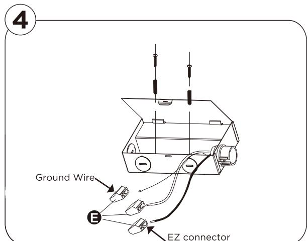
4. Open the connectors box cover. Feed supply wire into knockout hole using connector and make all connections inside the junction box using the EZ connectors (see picture below). Connect the 120V line wire to the black wire. Connect the neutral wire to the white wire. Connect ground wire with bare cooper wire. Put on junction box cover.
