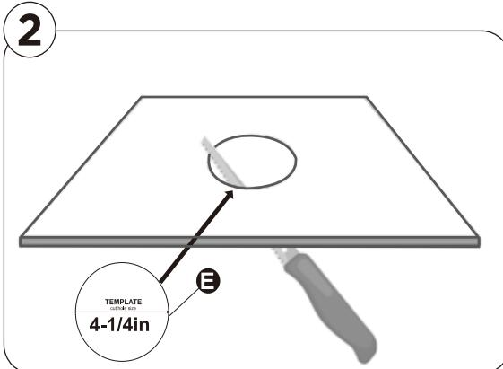
2. Make a hole in the ceiling with template in package
