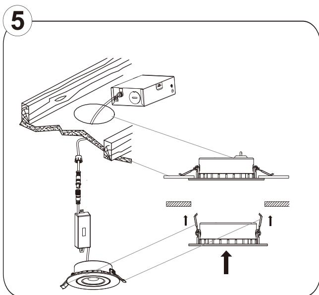
5. Connect male and female cable, raise spring evenly and push light kit into ceiling hole.
