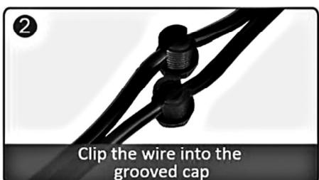
Clip the wire into the grooved cap
