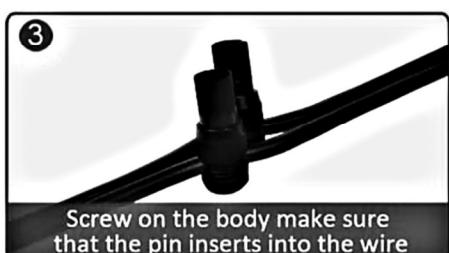
Screw on the body make sure that the pin inserts into the wire
