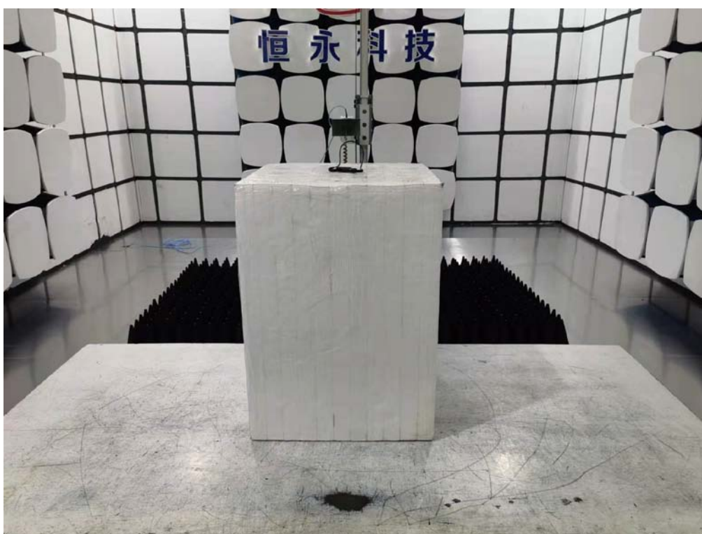
Radiated emission test: Above 1GHz
