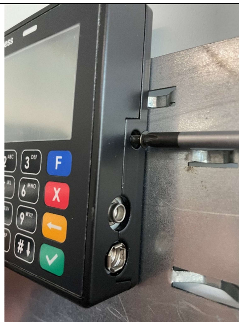
6. Screw the bolt you kept (check step 2) back firmly.
