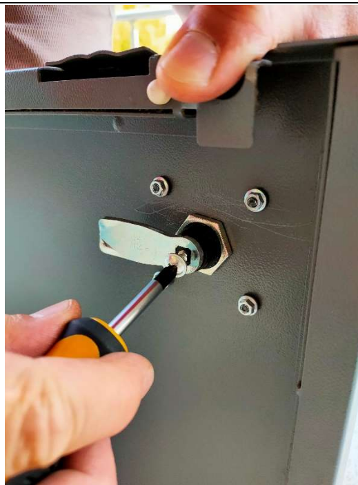
8. Fit the lock fixing plate on the front. Secure the plate with M4 nuts from the back. Insert the lock
