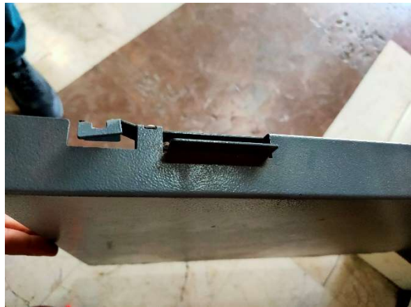
2. Bent the protruding parts with pliers so that the surface is plain
