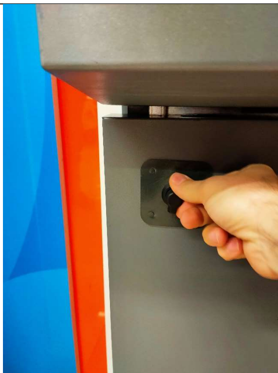
8. Fit the lock fixing plate on the front. Secure the plate with M4 nuts from the back. Insert the lock
