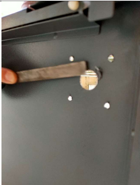
5. Clean the holes from inside
