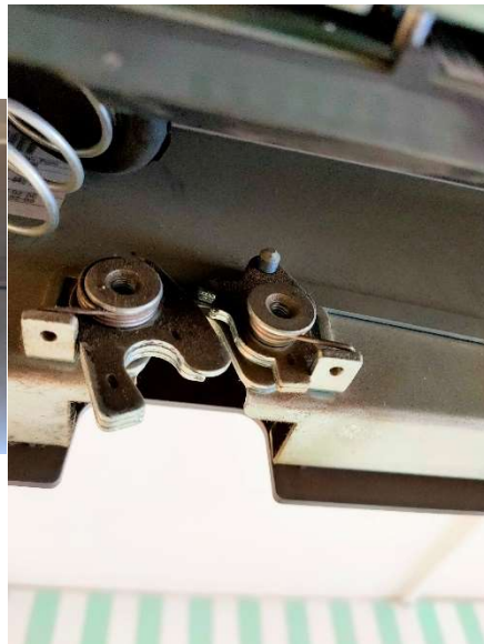
1. Remove the lock rings and bolts from the door
