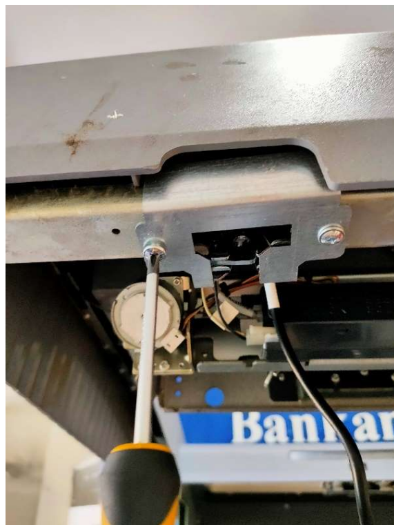
5. Fix the plate with M4x12 RYSB bolts. Install the nut from the inside
