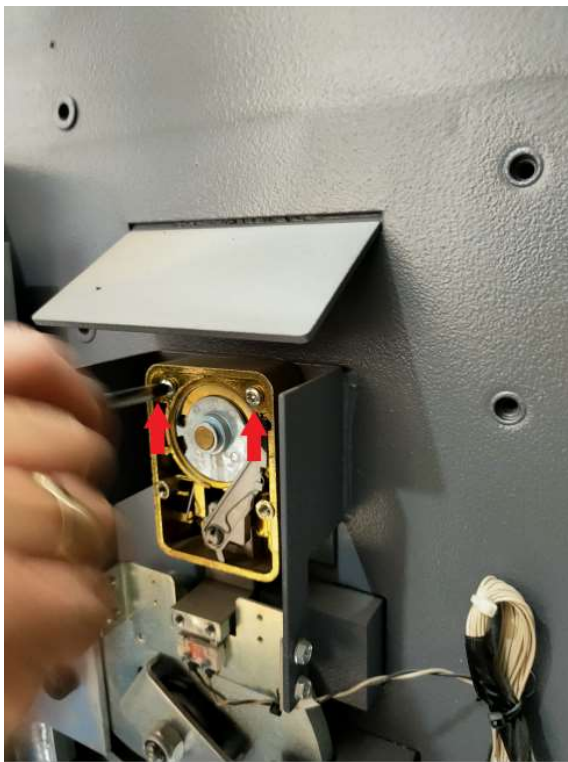
5. After removing the cover, unscrew the existing lock.
