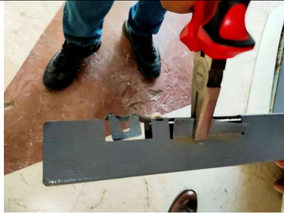
2. Bent the protruding parts with pliers so that the surface is plain
