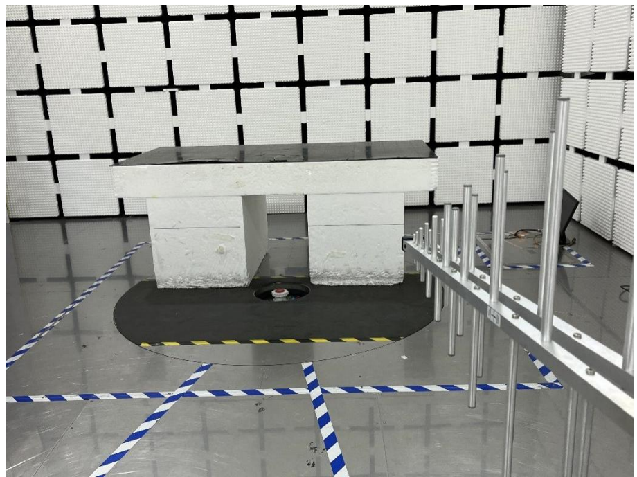
Radiation Emission Test Setup (30MHz to 1GHz)
