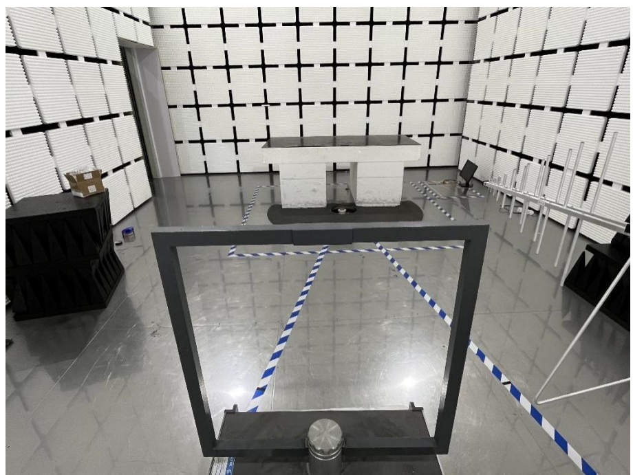
Radiation Emission Test Setup (Below 30MHz)
