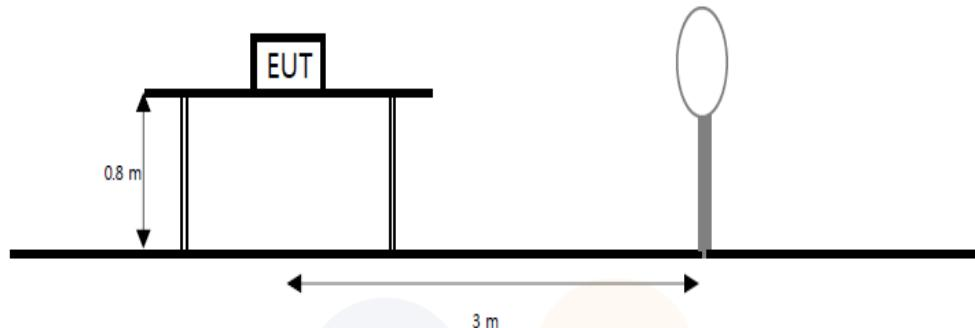
The diagram below shows the test setup that is utilized to make the measurements for emission from 30 MHz to 1 GHz emissions.
