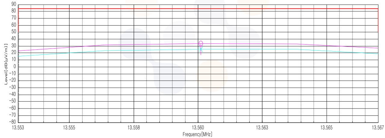
**Test results for in-band & out-band (9 kHz to 30 MHz)****15.225 (b,c) 13.110-14.010 MHz**
