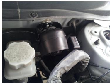
Step 3: connect the red cable to engine battery +, and connect the black cable to engine battery -, and sort out the left cables.
