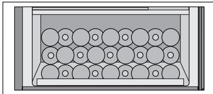
The wooden bottom bottle rack is intended for storing the bottles in the compressor area. This area is suitable for storing bottles you wish to keep for a longer period of time, especially for ageing without excessive vibration and unnecessary movement. Up to 27 Bordeaux bottles (25.4 fl oz (0.75 l)) can be stored on the wooden bottom bottle rack.
