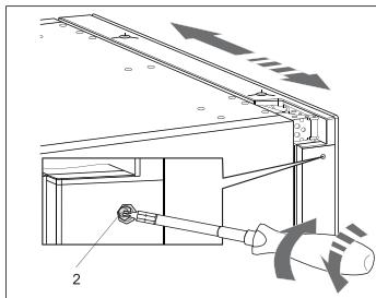
3. Close the door, then rotate the screw (2) at the top and bottom to adjust the door position.
