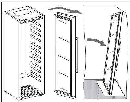
4. Remove the door, complete with the hinges, by moving it in the direction indicated by the arrow. Carefully place the door on the surface prepared for this purpose.
