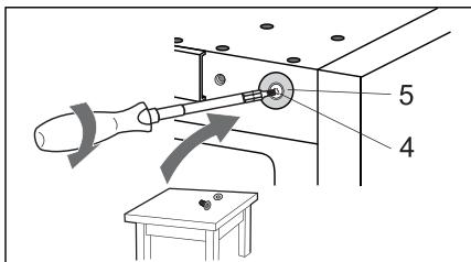
13. On the opposite side from the top hinge, attach the cap (5) using the screw (4).
