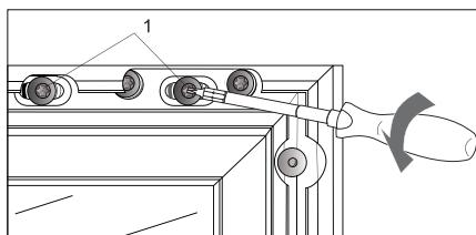
2. Release the screws (1) at the top and bottom. Do not undo them completely!
