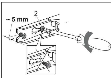
3. Partly (by no more than 5 mm) undo the hinge screws (2) at the top and bottom. Do not completely undo the screws. This way, the door will remain in contact with the housing.
