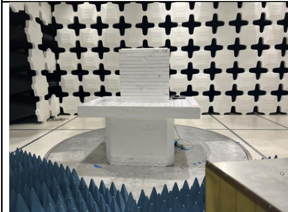
Radiated Emission Test above 1GHz Front View
