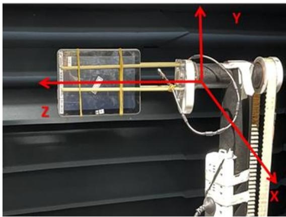
2. Antenna Field Pattern test, Ant2 test setup photo.
