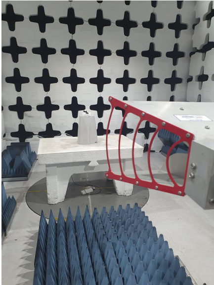
Radiated emissions test set up above 1GHz.
