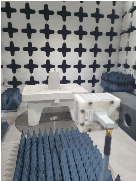
Radiated emissions test set up above 18GHz.
