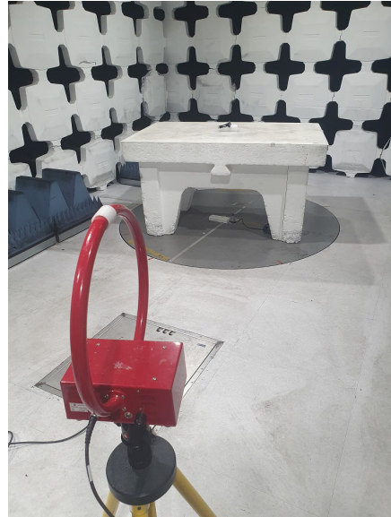
Radiated emissions test set up below 30MHz.
