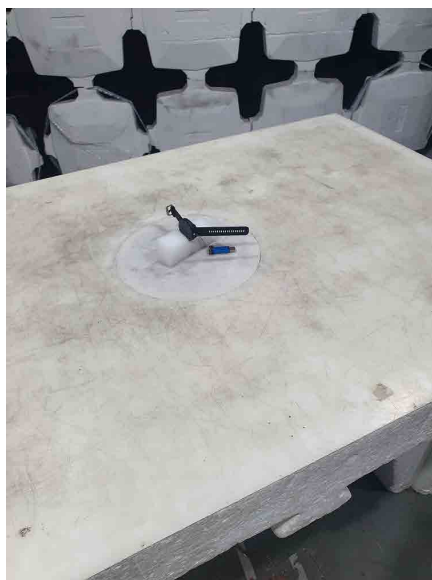
Picture 1 Radiated spurious emission test setup below 1 GHz
