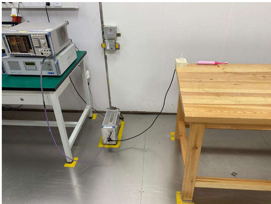
Conducted Emissions Test Setup
