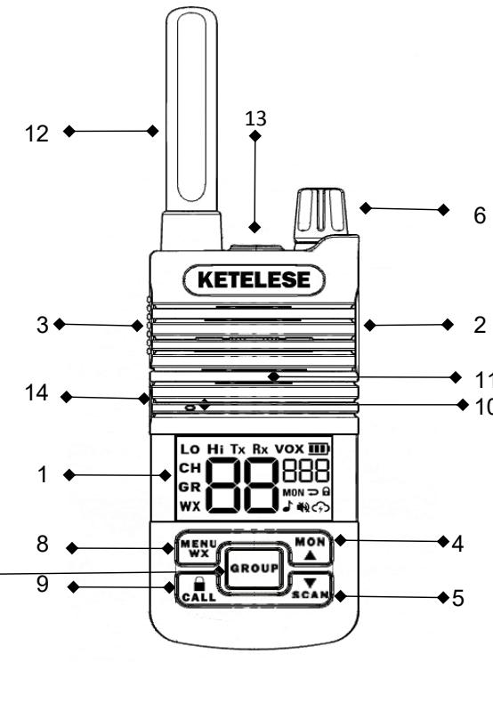
● **GROUP** Button – Enable the radio transmitting on GROUP-channel which is different from the PTT-channel.
