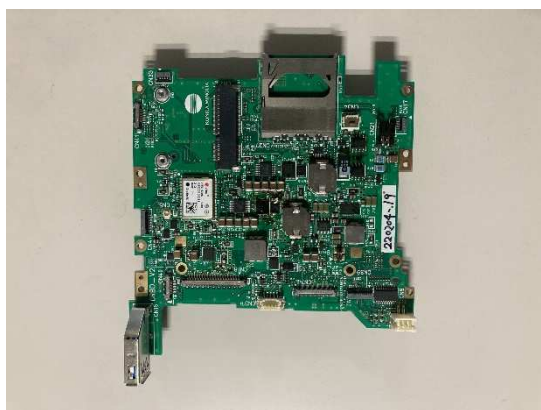
PCB Removing Seal and RF Module
