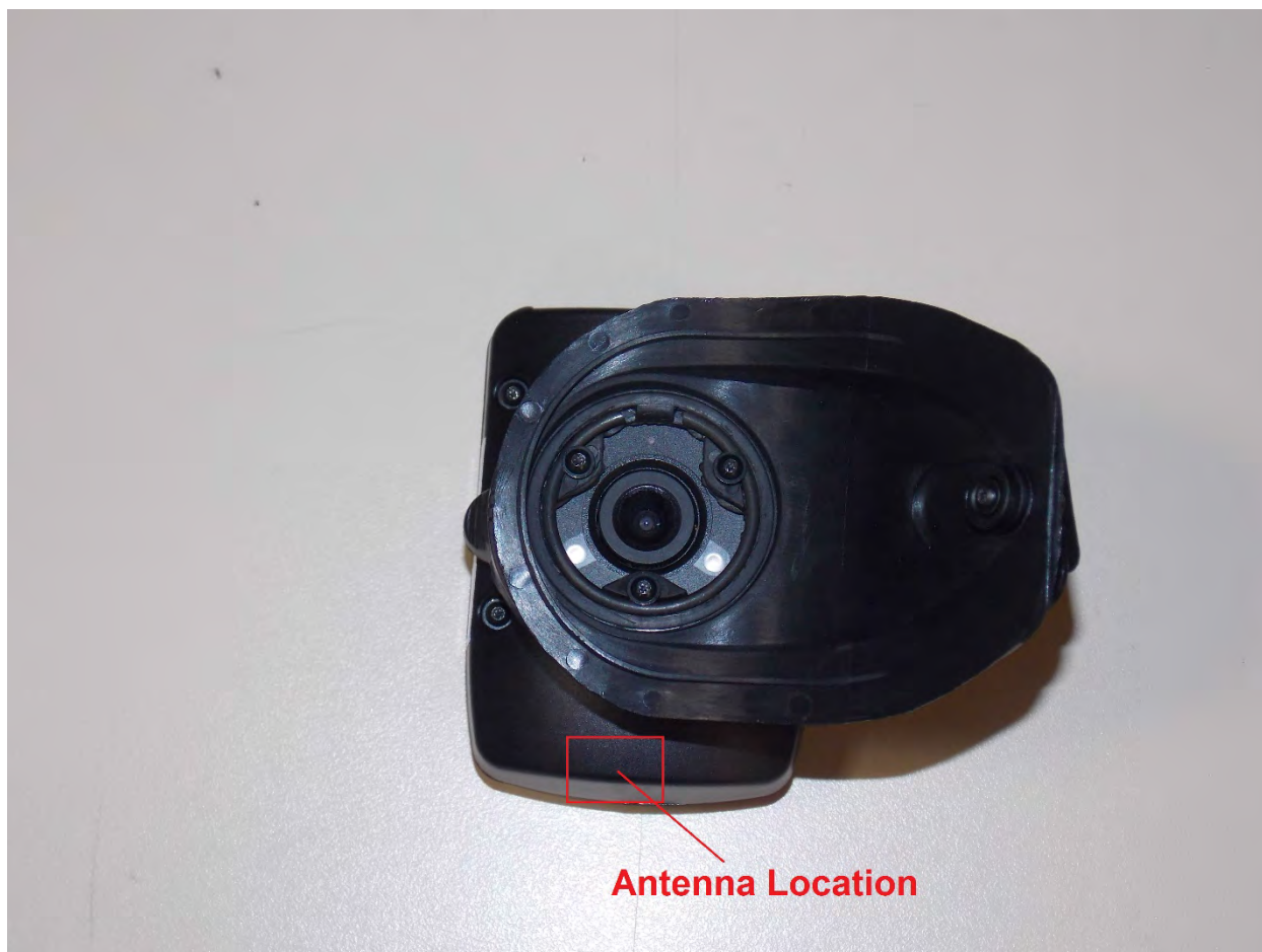
Antenna Location in Camera Unit
