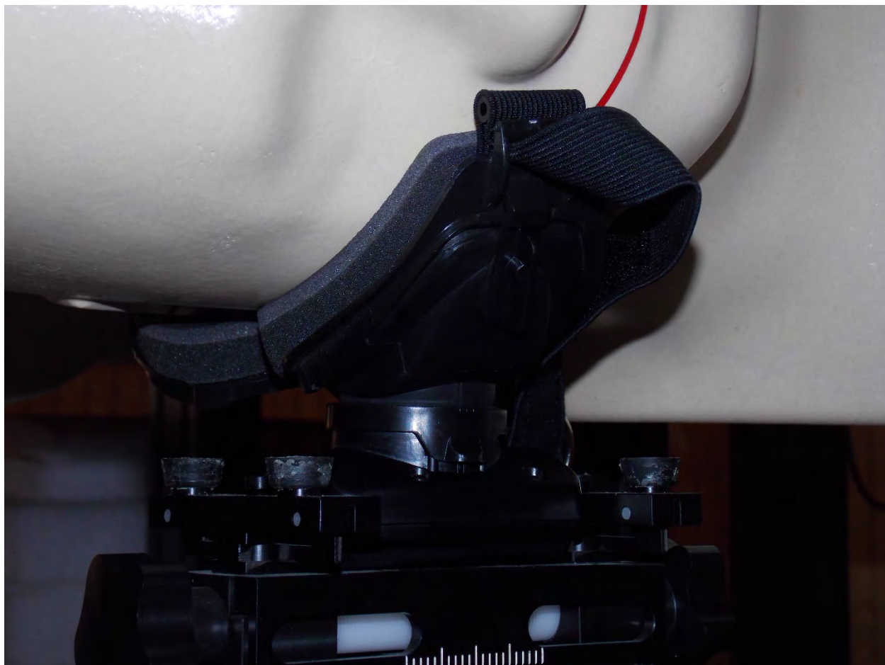
Proposed Test Position on SAM Phantom Side View of Device
