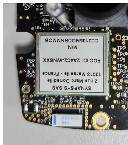
View of the electronic board from (patient's side), with a zoom on the radio module and the antenna
