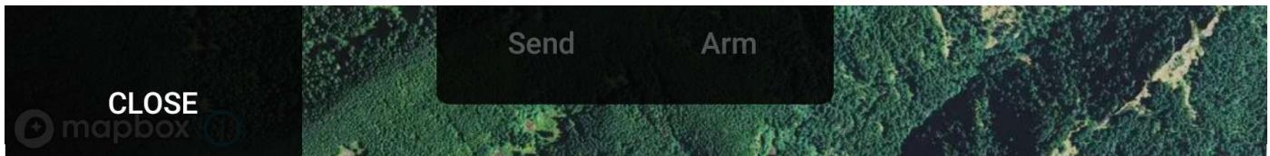
Click one, and a panel containing `Send` and `Arm` buttons will appear. Click `Send` and the mission will be generated and sent to the vehicle. At that point, the `Arm` button can be used to arm the motors. Once you've done that: If your mission has a `Takeoff` point, you can click `Start` and the mission will start on its own. Otherwise, you can click `Takeoff`, and then `Start`. Alternatively, you can launch manually, and then click `Start`.
