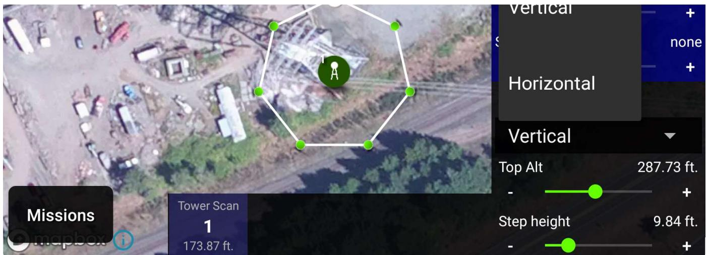
A Vertical scan starts at the base altitude of a scan leg and flies straight up to the top of the leg. Once there, it moves over to the next leg, and flies straight down to the base altitude. It continues this pattern until the end of the scan. If you have "Take Picture" turned on, it stops at intervals on the way up or down and takes a picture.
