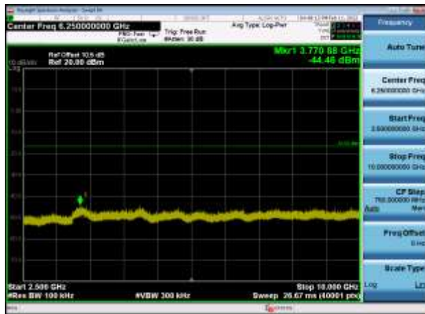
Plot 4,2500MHz~10000MHz-802.11g ,2462MHz,Ant0
