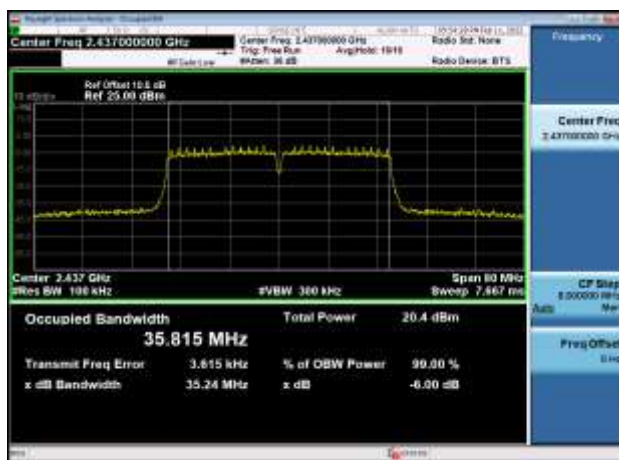
6dB Bandwidth-802.11n(HT40),2437MHz ,Ant0
