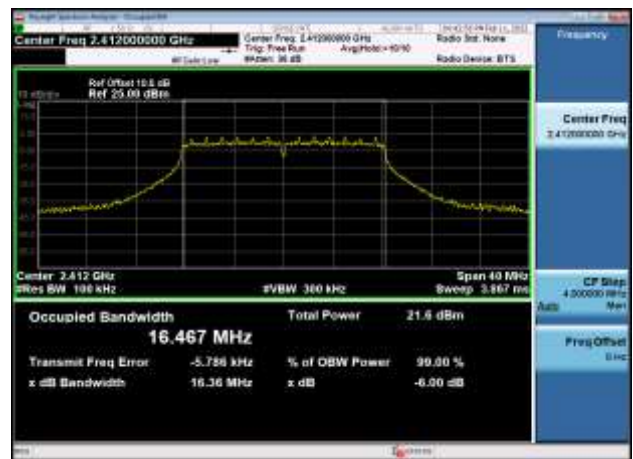
6dB Bandwidth-802.11g,2462MHz,Ant0
