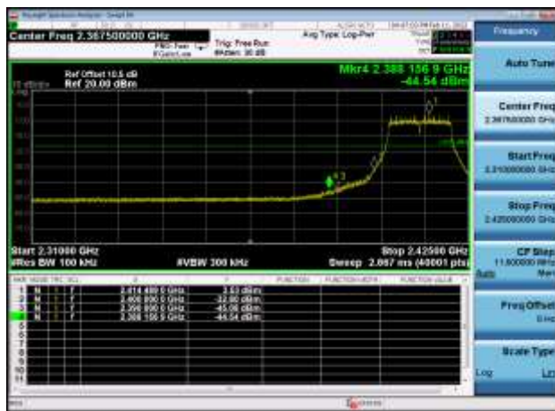
Plot 2,Band Edge-802.11g,2462MHz ,Ant0
