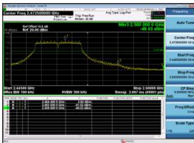
Plot 3,30MHz~2310MHz-802.11g,2437MHz ,Ant0
