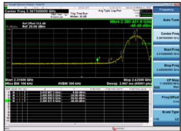
Plot 2,Band Edge-802.11b,2462MHz ,Ant0
