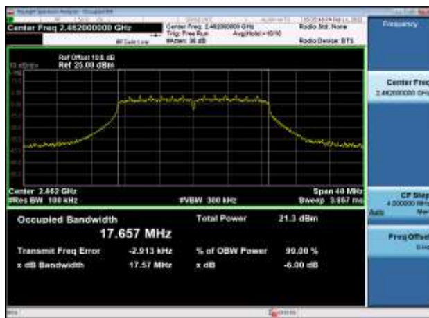
6dB Bandwidth-802.11n(HT40),2437MHz ,Ant0
