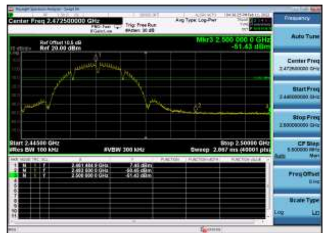
Plot 2,Band Edge-802.11b,2462MHz ,Ant0
