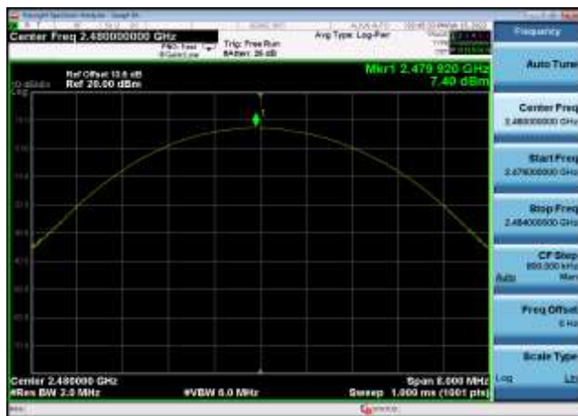
Output Power: 8DPSK,2480MHz,3DH5
