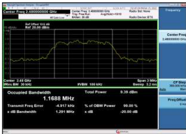
20dB Bandwidth: 8DPSK,2480MHz,3DH5
