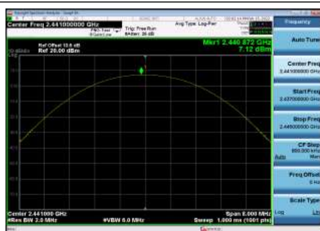
Output Power: DQPSK,2441MHz,2DH5
