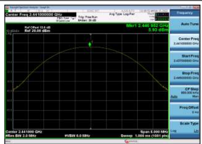
Output Power: DQPSK,2402MHz,2DH5
