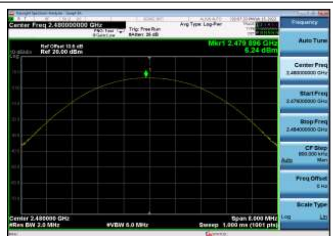
Output Power: DQPSK,2480MHz,2DH5
