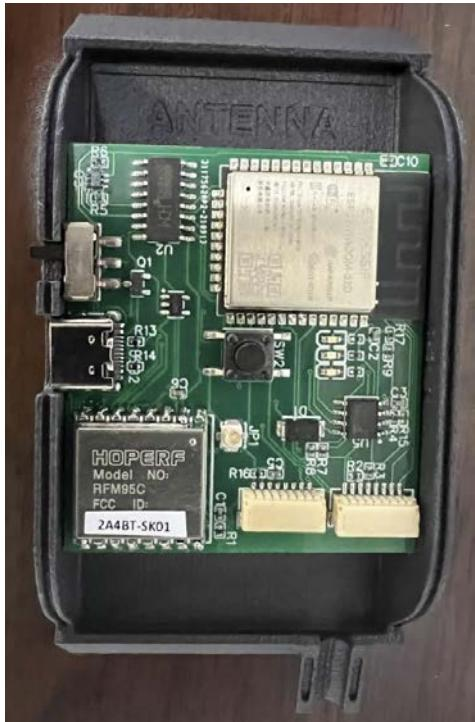
Prior to final assembly of the lid enclosure, all of the PCB assemblies containing an RFM95C chip must be inspected for quality control to confirm that the label has been properly affixed.
