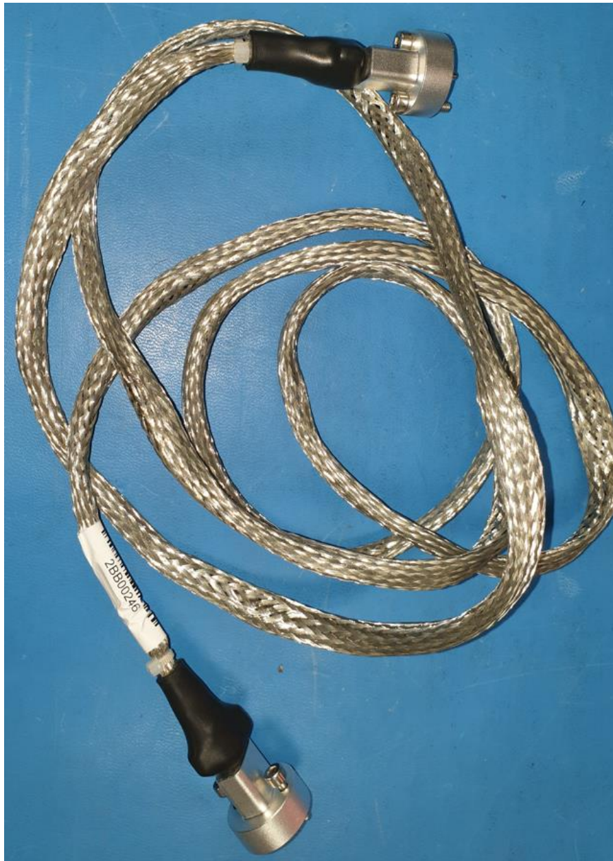
Figure 10 – Cable assembly that connects the TN001XC to the TN201SP
