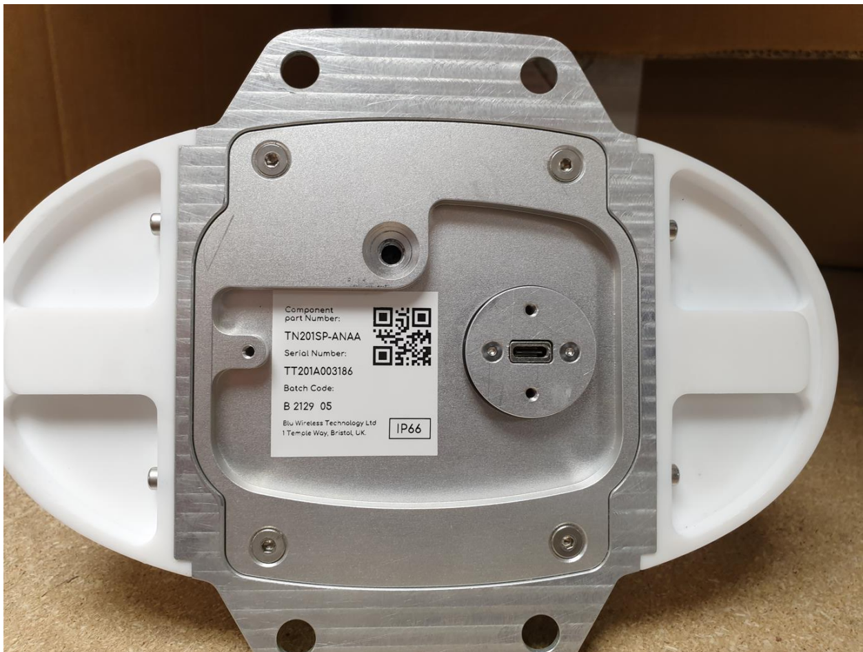
Figure 6 – TN201SP bottom view, showing example label and mounting holes
