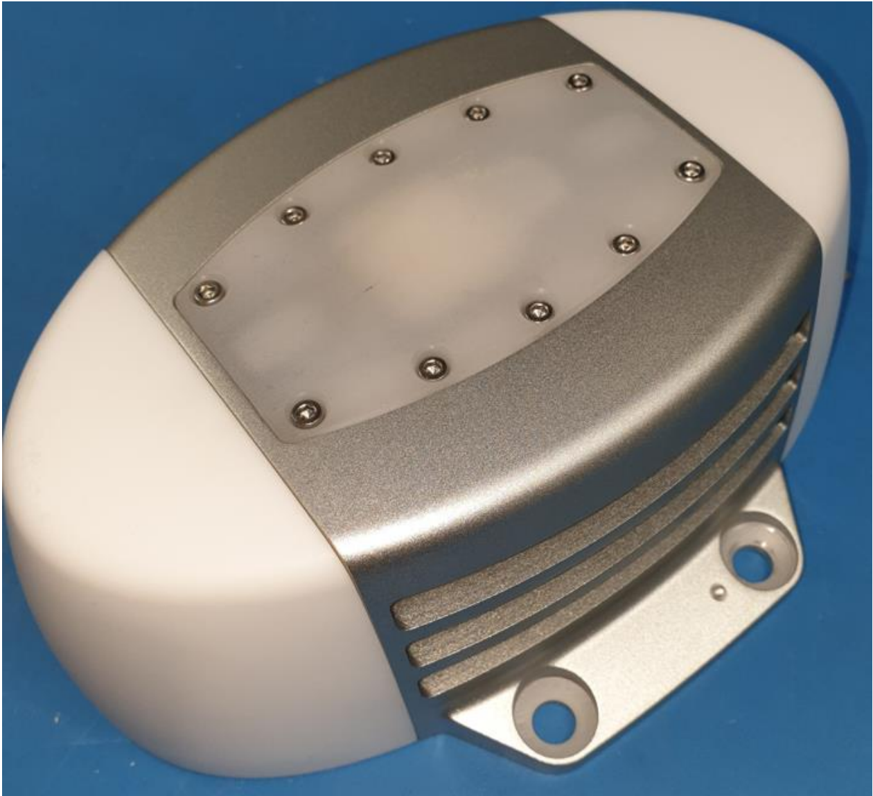
Figure 5 – TN201SP top and side view, showing the two RF radomes and the GPS radome on top
