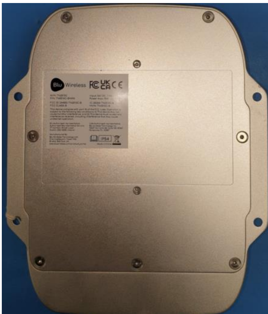
Figure 4 – TN001XC back view showing an example label and the bracket mounting holes
