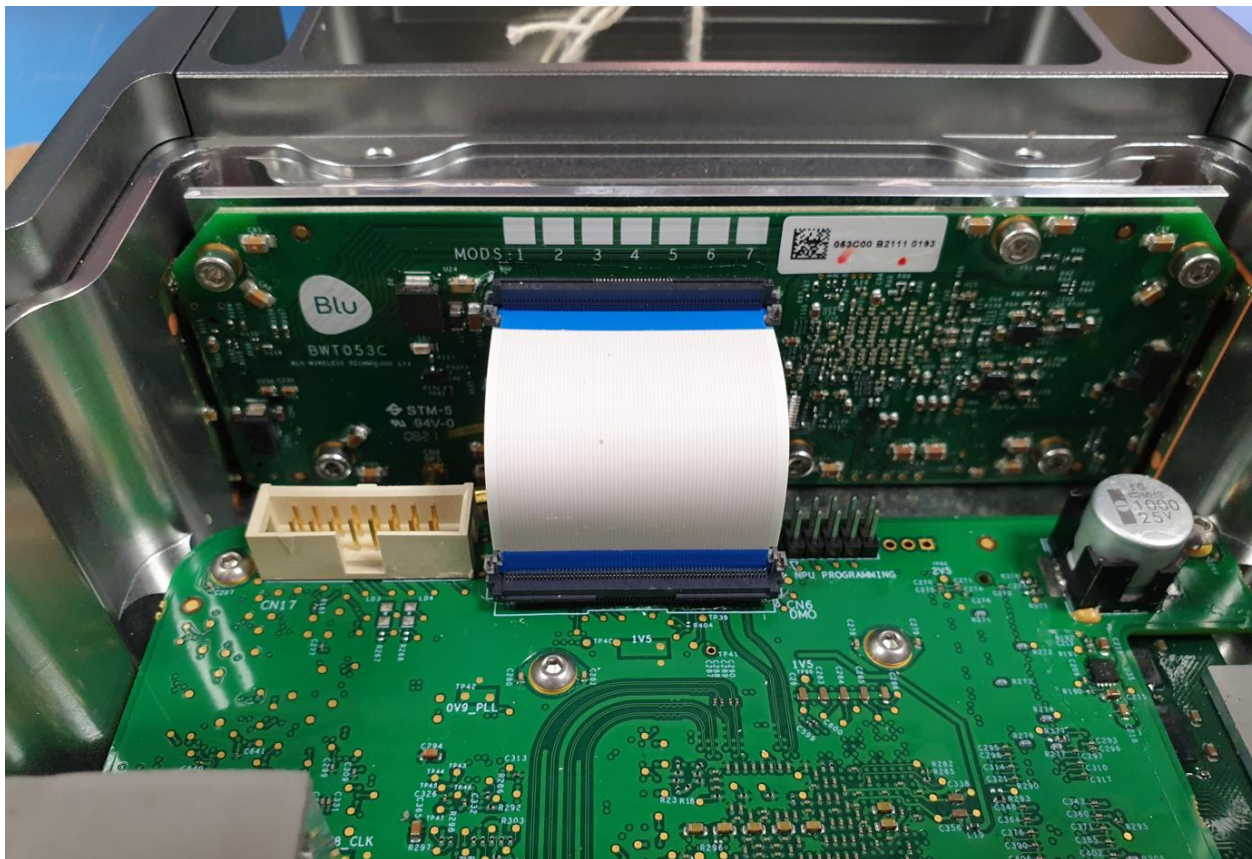
Figure 3 – Inside Back cover of DN201SC showing the BWT053 Modem board connected to the processor board via FFC
