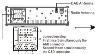
When connecting the speakers. The speakerwires +/- must be connected with the speaker +/- directly. Any speaker wire can't connect with the iron or ground. Otherwise the unit may be damaged.
