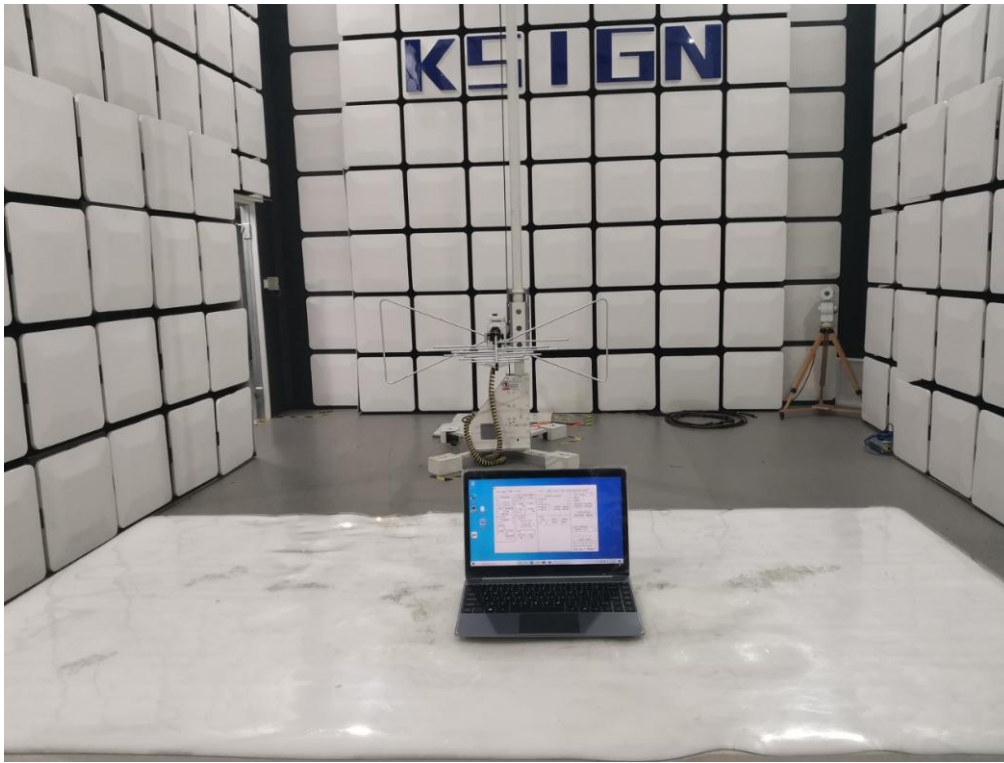
Radiated Measurement (Above 1GHz)
