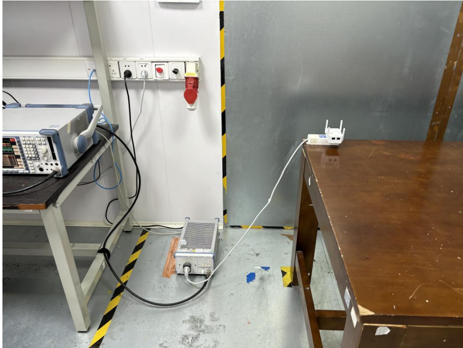
Conducted emissions at AC power line (150kHz-30MHz)
