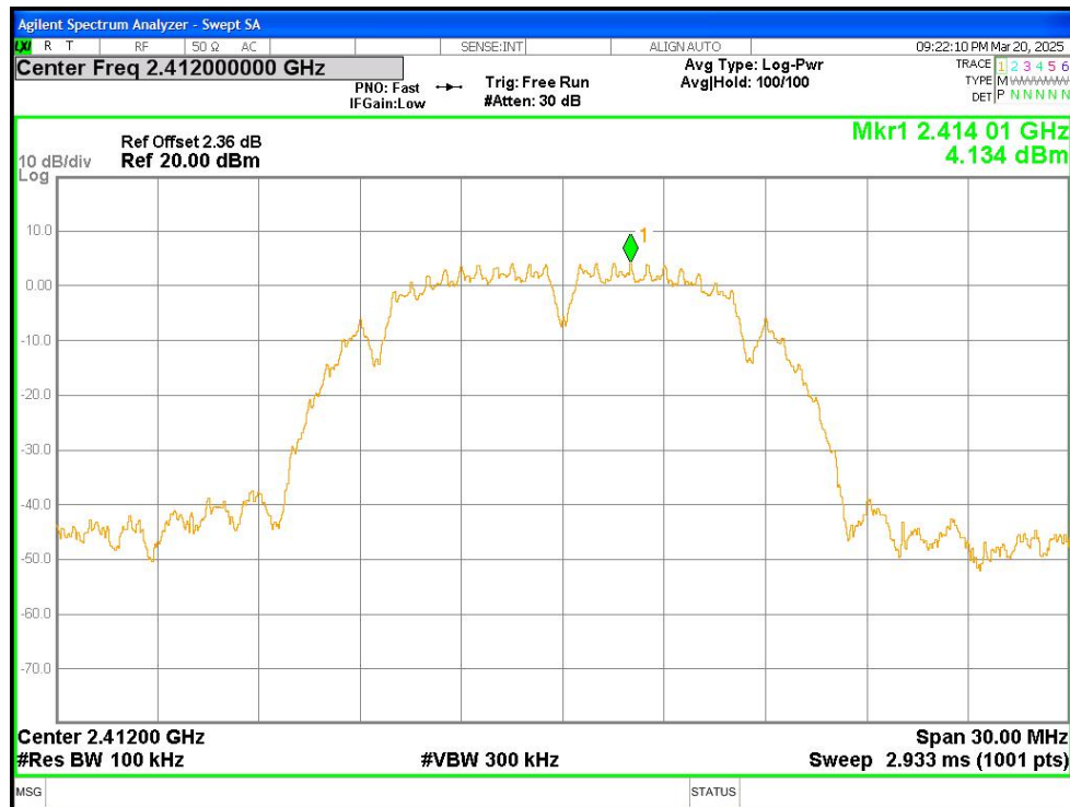
Band Edge NVNT b 2412MHz Ant1 Emission
