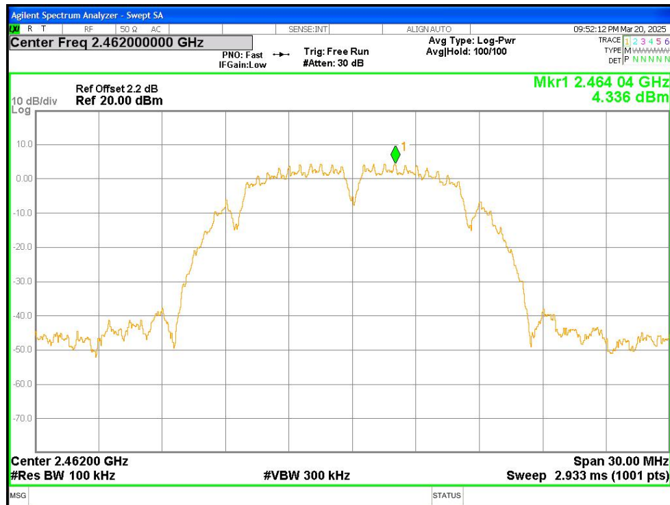
Band Edge NVNT b 2462MHz Ant1 Emission
