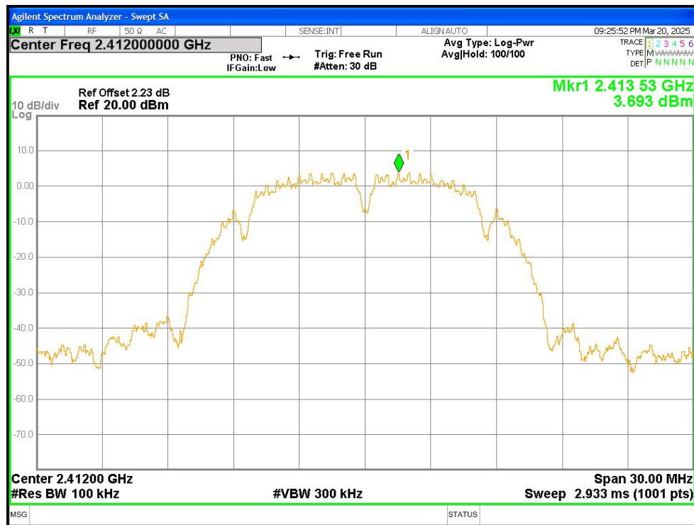
Band Edge NVNT b 2412MHz Ant2 Emission
