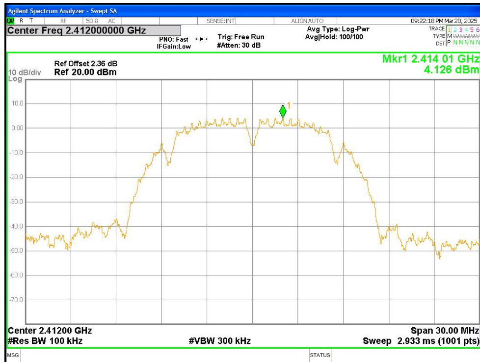
Tx. Spurious NVNT b 2412MHz Ant1 Emission
