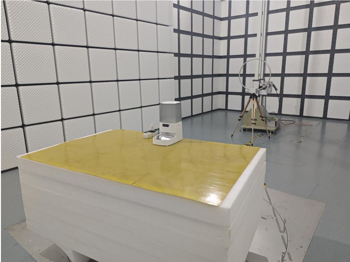
Radiated Spurious Emissions Test View (9kHz-30MHz)
